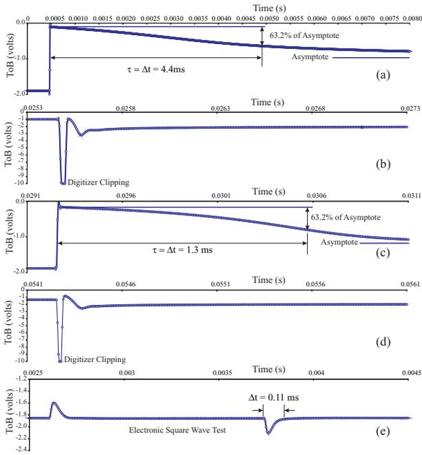
Figure 3: Severe transients and nonlinear response to  $RR$  for zero velocity conditions using a single additional balance resistor switched at 40 Hz : (a) Switch-On: 14.8% reduction in  $RR$ ,  $\tau \approx 4.4$  ms; (b) Switch-Off: 14.8% increase back to  $RR = 1.7$ ; (c) Switch-On: 7.7% reduction in  $RR$ ,  $\tau \approx 1.3$  ms; (d) Switch-Off: 7.7% increase back to  $RR = 1.7$ ; (e) Conventional electronic square-wave test (without  $RR$  switching).
