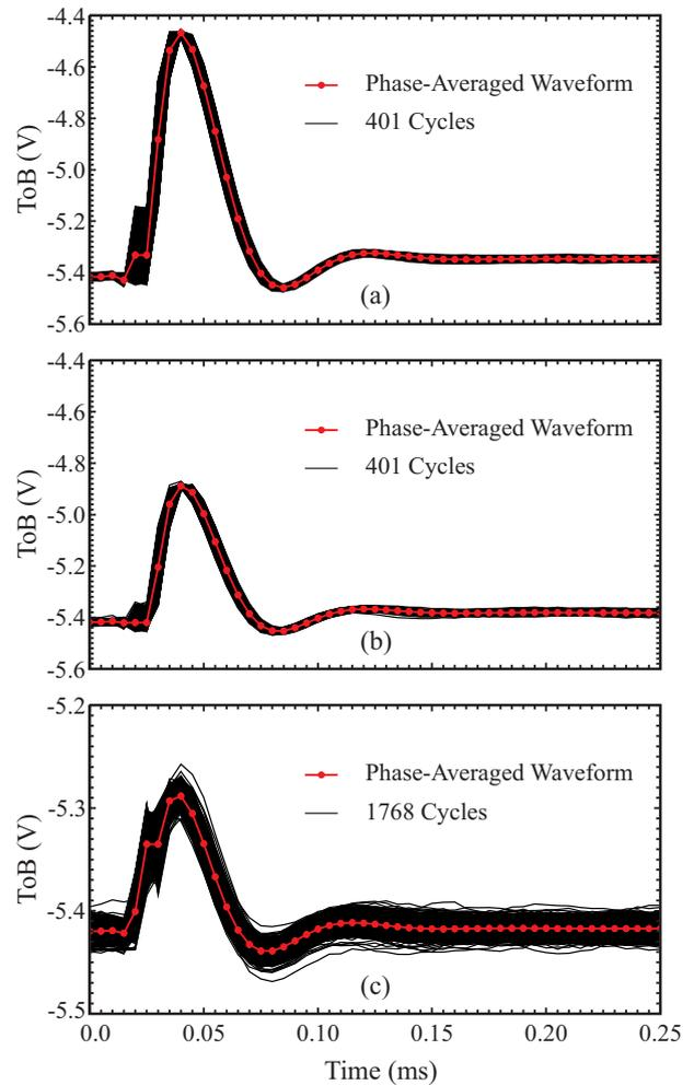
Figure 6: Small amplitude  $RR$  switching. Hot-wire signals at  $M = 0.5$ ,  $\rho.U = 200$  kg/s operating at  $RR = 1.833$  with dynamic switching at 200Hz to (a)  $RR = 1.813$  (-1%), and (b)  $RR = 1.796$  (-2%). Data sorted into 401 cycles (solid black curves) and phase-averaged using 999 phase intervals. (c) Electronic square-wave test: Data sorted into 1768 individual cycles and phase-averaged on the basis of a signal transition threshold of 0.05 V between samples.
