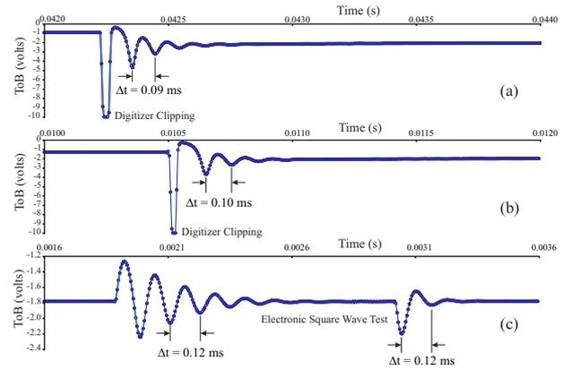
Figure 4: Detuned system. Response to  $RR$ , zero velocity, single additional balance resistor switched at 40 Hz : (a) Switch-Off: from a 14.8% reduction back to  $RR = 1.7$ ; (b) Switch-Off: from a 7.7% reduction back to  $RR = 1.7$ ; (c) Conventional electronic square-wave test (without  $RR$  switching).
