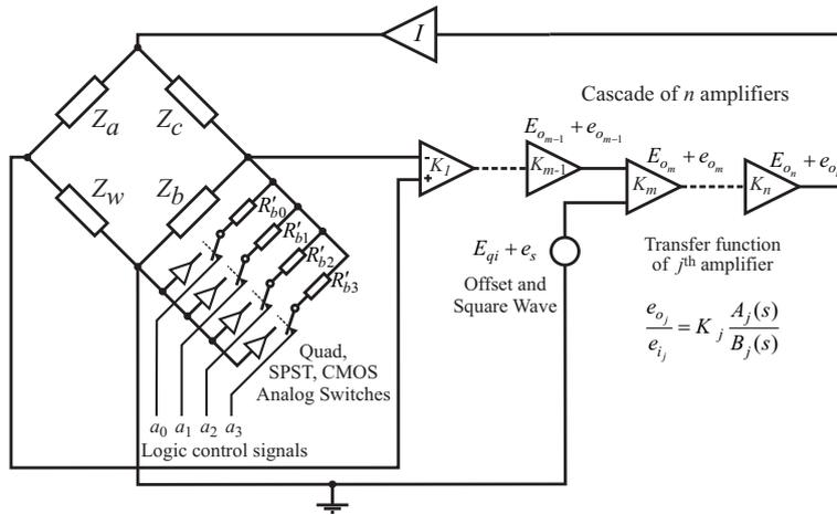
Figure 1: Schematic of constant-temperature hot-wire anemometer with four remote controlled CMOS analog switches for connecting additional resistors in parallel across the balance resistor,  $R_b$ , to allow high frequency multiplexing of Resistance Ratio.
