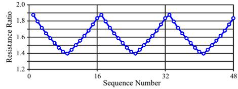
Figure 2: Alternate values of the ordered switching sequence used to obtain small step-size resistance ratio variations using the nearest available standard resistor to a geometric series. Three cycles of the sixteen resistance ratios are shown.
