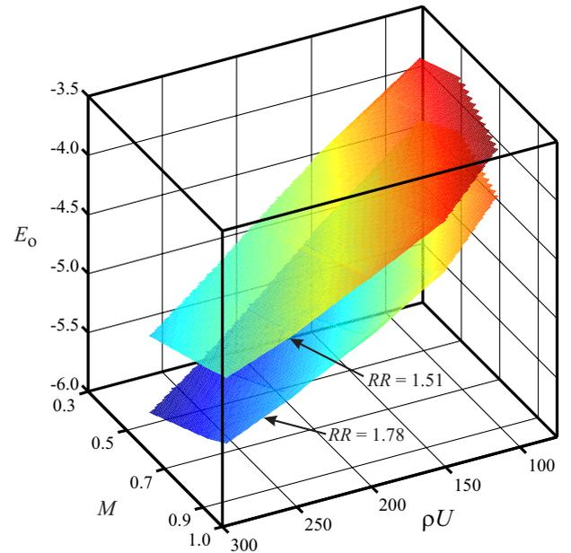
Figure 5: Static hot-wire calibration data performed in the DSTO Transonic Wind Tunnel using a 5 micron diameter, 1 mm long tungsten hot-wire filament manually switched between  $RR = 1.51$  and  $RR = 1.78$ .
